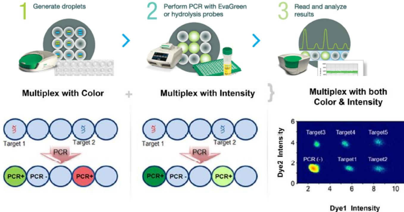
The Biorad Qx200-droplet-digital-PCR system
